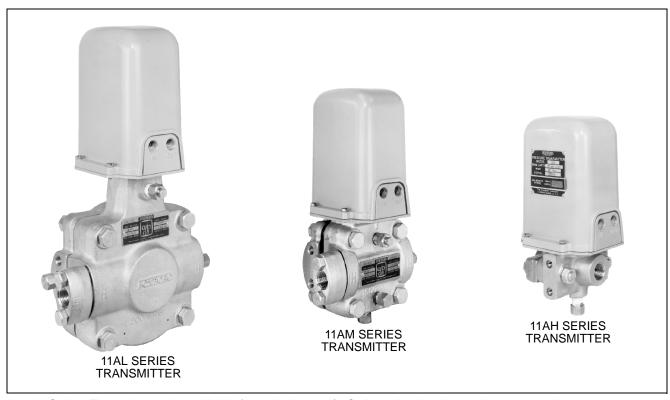
In 11A Series Transmitters, the reliable force-balance d/p Cell mechanism is used to accurately measure absolute pressure and transmit a standard pneumatic signal to nearby or remote receivers.
