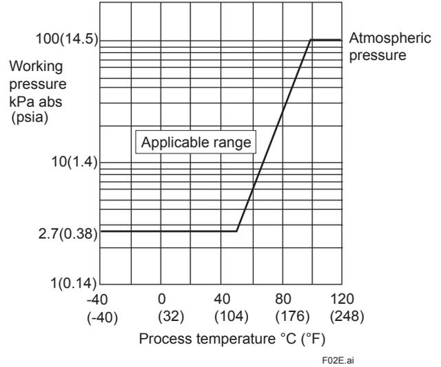
**Figure 1-2. Working Pressure and Process Temperature [For EJX530A]**
