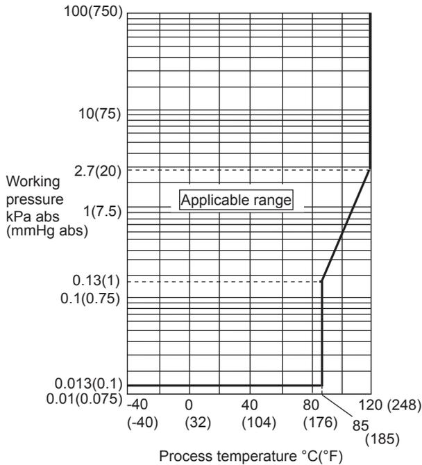
**Figure 1-1. Working Pressure and Process Temperature [For EJX510A]**
